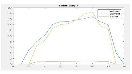
Hourly solar measurement variation of proposed real time System for Thursday Mar 12th, 2020. The horizontal line shows the time from 6:00 am to 7:00 pm, the time frame of 14 hour
