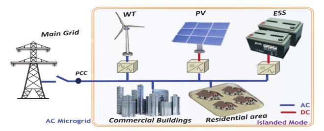
Fig. 1.1: The solar and wind power systems in AC load system
