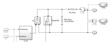
Figure 3: Simulink PV model [11]
