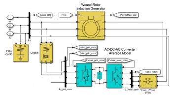
Figure 5: Modelling of wind turbine [11]
