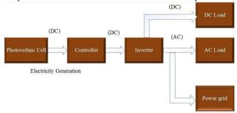
Figure 2: Schematic diagram of photovoltaic system
