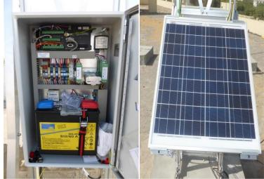
Fig. 6: Control box with data logger, battery and electric equipment Fig. 7. Solar panel [22]
