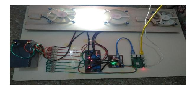
After the successful completion of first transaction we can see the load of Mr. Asad's house (in the center of the others loads) is receiving electricity for the time period of one minute because he has paid amount of three rupees that is the cost of one unit in our case.
